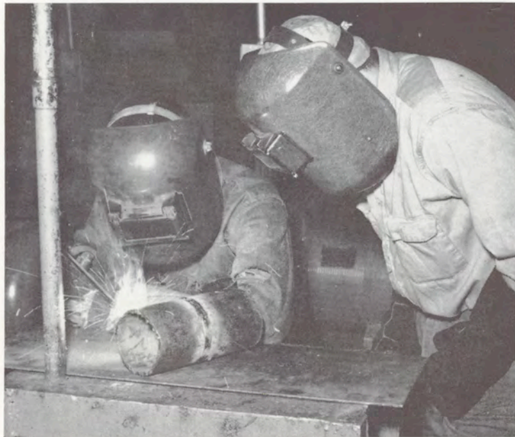
THE WELDING COURSE includes gas welding, burning, arc welding, and class work with emphasis upon "Learning by Doing." Students build welded projects and do actual repair work. Welding in the picture above are James Hathaway and Jim Garbett.
