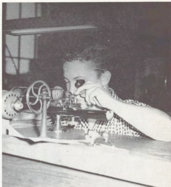
THE WATCHMAKING DEPARTMENT gives the basic fundamentals in one of the oldest trades. Upon completion of this course the student should be thoroughly familiar with the correct methods and procedures of good watchmaking. Bruce Haugen, a Junior, is shown above cutting a winding stem.
